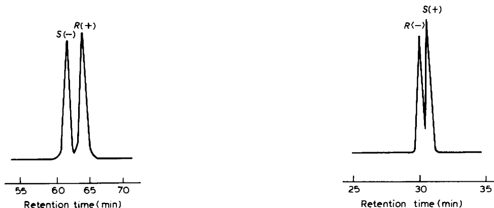
Fig. 1. Gas chromatogram of racemic O-acetyl-1-phenylethanol. Glass capillary column (40 m \times 0.25 mm I.D.) coated with N-(1 R ,3 R )- trans -chrysanthemoyl-( R )-1-( \alpha -naphthyl)ethylamine. Temperature: 80°C. Carrier gas: helium at a flow-rate of 0.7 ml/min.
